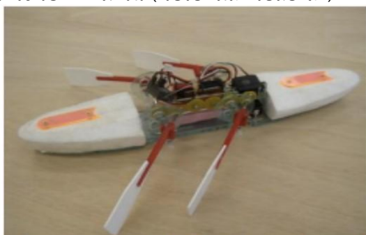
Servo motor 1: for backwards and forwards movements
