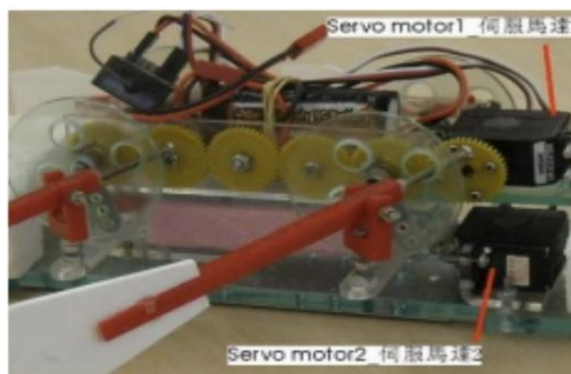
Servo motor 2: for left or right turns
